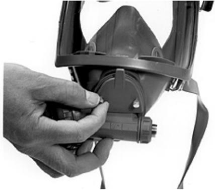
3. Turn the breathing valve clockwise so that it comes away from the bayonet fitting and pull the valve outwards.
