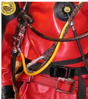
Examples of relieving loop attachment to the life belt
