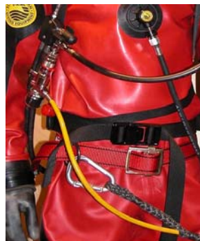
Examples of relieving loop attachment to the life belt
