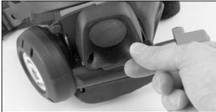
3. Connect the breathing valve to the medium pressure supply hose and the by-pass unit. The locking sleeve of the female quick coupling will automatically move forward and snap into place, locking the breathing hose in place.
