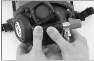
2. Lock it into position by sliding down the outer speech cone and tighten the screw by hand. In the correct position the serial number on the breathing valve is covered by the lip of the speech cone.
